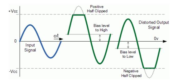
For a signal amplifier to operate correctly without any distortion to the output signal, it requires some form of DC Bias on its Base or Gate terminal. A DC bias is required so that the amplifier can amplify the input signal over its entire cycle with the bias "Q-point" set as near to the middle of the load line as possible.
