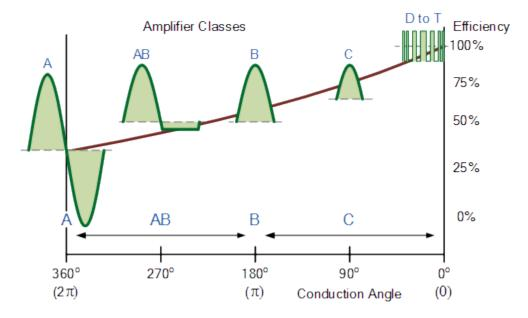
As well as audio amplifiers there are a number of high efficiency **Amplifier Classes** relating to switching amplifier designs that use different switching techniques to reduce power loss and increase efficiency. Some amplifier class designs listed below use RLC resonators or multiple power-supply voltages to reduce power loss, or are digital DSP (digital signal processing) type amplifiers which use pulse width modulation (PWM) switching techniques.
