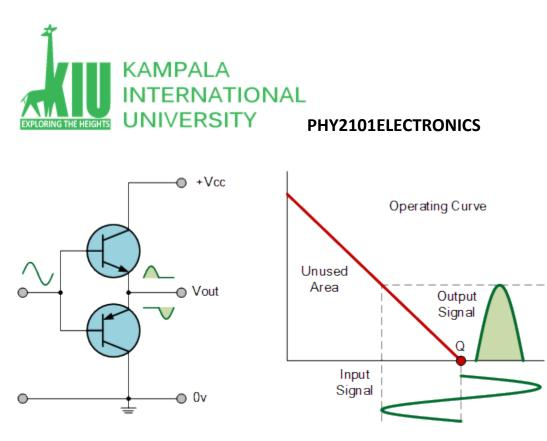
When the input signal goes positive, the positive biased transistor conducts while the negative transistor is switched "OFF". Likewise, when the input signal goes negative, the positive transistor switches "OFF" while the negative biased transistor turns "ON" and conducts the negative portion of the signal. Thus the transistor conducts only half of the time, either on positive or negative half cycle of the input signal.
