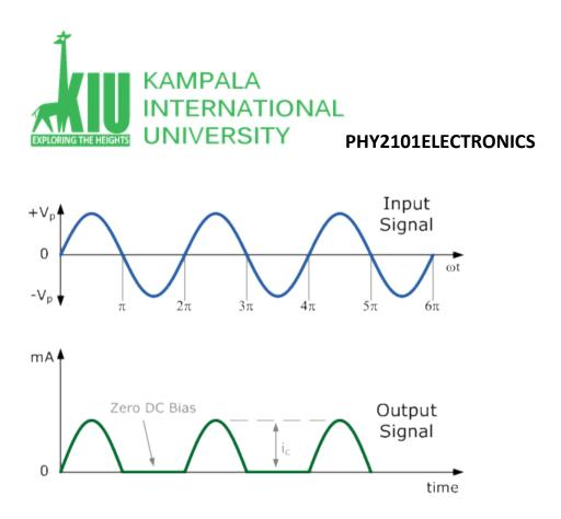
In a Class-B amplifier, no DC voltage is used to bias the transistors, so for the output transistors to start to conduct each half of the waveform, both positive and negative, they need the base-emitter voltage  $V_{BE}$  to be greater than the 0.7v forward voltage drop required for a standard bipolar transistor to start conducting.
