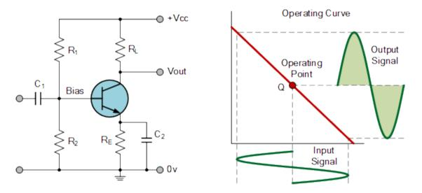
To achieve high linearity and gain, the output stage of a class A amplifier is biased "ON" (conducting) all the time. Then for an amplifier to be classified as "Class A" the zero signal idle current in the output stage must be equal to or greater than the maximum load current (usually a loudspeaker) required to produce the largest output signal.
