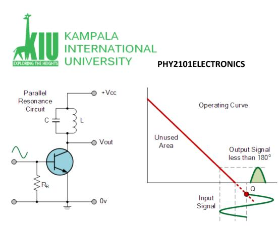
Due to its heavy audio distortion, class C amplifiers are commonly used in high frequency sine wave oscillators and certain types of radio frequency amplifiers, where the pulses of current produced at the amplifiers output can be converted to complete sine waves of a particular frequency by the use of LC resonant circuits in its collector circuit.
