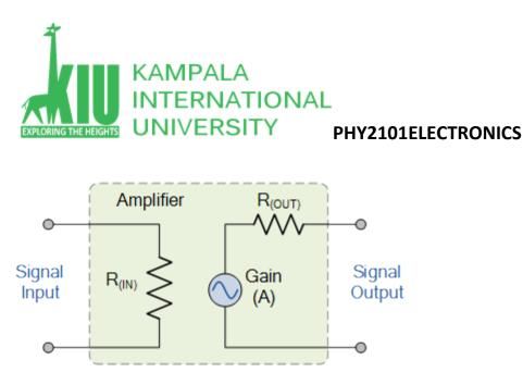
The amplified difference between the input and output signals is known as the Gain of the amplifier. Gain is basically a measure of how much an amplifier "amplifies" the input signal. For example, if we have an input signal of 1 volt and an output of 50 volts, then the gain of the amplifier would be "50". In other words, the input signal has been increased by a factor of 50. This increase is called **Gain**.
