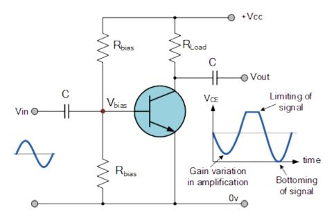
Distortion of the output signal waveform may occur because:
