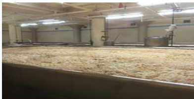
Open vessel showing fermentation taking place
