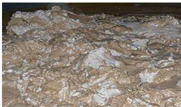
A mixture of diatomaceous earth and yeast after filtering
