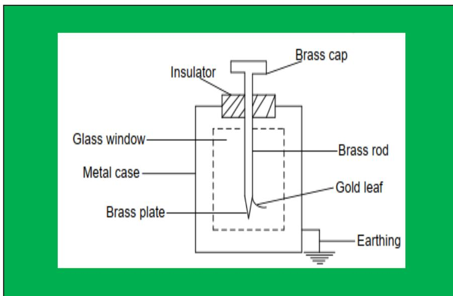
The electroscope is charged negatively by touching the brass cap with a negatively charged amber rod
